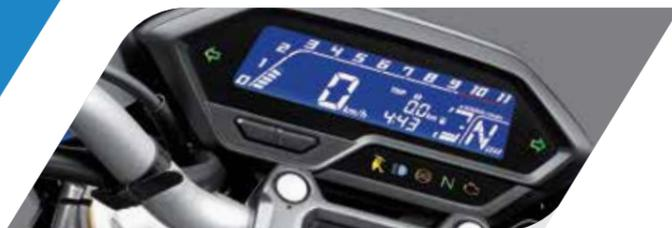
The perfectly positioned meter lets you know exactly how fast you're going as you assert your dominance. Be it night or day, see your info clearly with the 5-level Illumination Control on the crystal meter. Also, with the Gear Position Indicator, Battery Voltmeter and Service Due Indicator, stay above the rest. It also includes the Side Stand Indicator with Engine Cut Off that adds to the safety of the rider, indicating when the stand is down.
